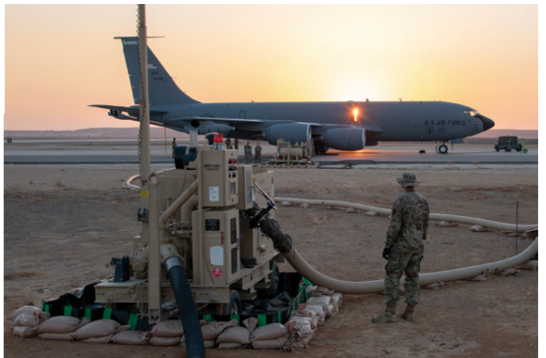
U . S. Air Force Staff Sgt. Munoz, 332nd Expeditionary Logistics Readiness Squadron, refuels a KC-135 Stratotanker with a force system at an undisclosed location in Southwest Asia, Feb. 13, 2020. This new capability will provide more efficient and effective ground refueling. (U.S. Air Force photo by Staff Sgt. Alexandria Brun) ▲
